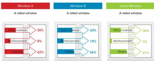
We know that Liniar profiles can be more expensive, per metre, than other PVCu systems. This is due to the patented innovations its products contain, as well as the modern machinery used to create them. The Liniar system is designed with reduced reinforcement and often requires a lower specification of glazing to reach high WERs and low U-values – both of which can contribute to overall cost savings when fabricating a window.
