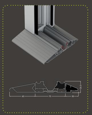
Low Threshold and Full Tray Threshold Height: 26.5mm
