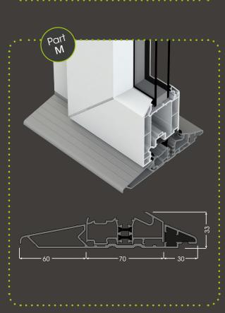
Low Threshold and Full Tray Threshold Height: 33mm
