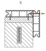
be within 30mm of the deck board edge to ensure trim coverage. necessary to screw at an angle into the sub-frame. The screw head must overhang (max 25mm), it may be If installing SwitchBoard with an
