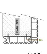
methods below. Fix down final board in position at 600mm (max) centres along the length of the board. See fixing
