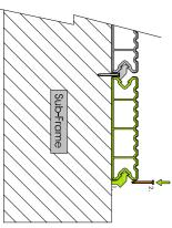
But the next board up to the clips and secure this board as shown in step 3. Repeat for all remaining boards.
